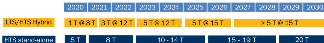
Figure 1 A list of milestones towards a dipole field of 20 T using REBCO conductors.
