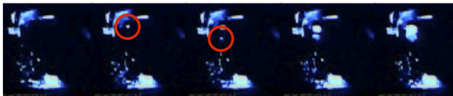
Fig. 1: Example of the formation of two merging snowballs, likely to be caused by the same neutron. There are 150 ms in between frames.
