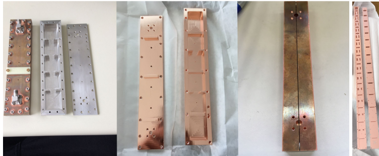
Figure 1: From left to right: first 5 sub-cavities structure with inductive couplings (non-tunable), alternating 6-cav structure (non-tunable), 5 sub-cavities vertical cut structure (tunable), alternating 30-cavities structure. The first three structures are each about 15cm long, the 4th one is of about approximately 1m length.
