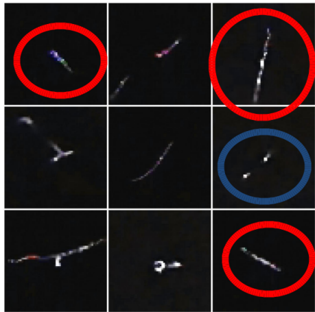
Figure: The variety of particle tracks candidates as registered by a smartphone using the CREDO Detector app.
