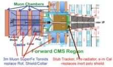
Cartoons (not fully to scales) of Lepton-Photon systems for the the CMS Forward Region only as an example: Passive regions that could be replaced with active devices
