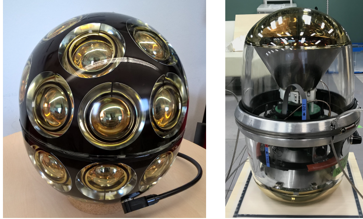
Figure 1: Prototypes of an mDOM (left) and an D-Egg (right) for the IceCube Upgrade.
