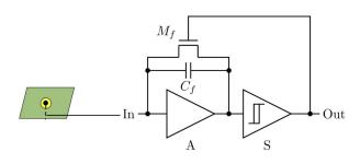
and returns the circuit to a stable baseline and the cycle is free to begin again. This ``reset" transition pulse is used to capture and store the current value of a local clock within one ASIC. This changes the basic quantum of information for each pixel from the traditional ``how much charge per unit time" to the difference between one clock capture and the next sequential capture, referred to as the Reset Time Difference (RTD). This new unit of information measures the time to integrate
