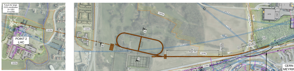
Figure 1: Overview of the proposed implementation of nuSTORM at CERN [1]. The fast-extraction system that will provide protons at 100 GeV to the nuSTORM target will be installed in LSS6 where an existing extraction system serves beam to the West Area. Beam will be transported through an existing transfer tunnel (TT60). Before TT60 enters the Meyrin site, the beam will branch into a new transfer tunnel. The nuSTORM ring will be sited between the West and North areas. The production straight illuminates a near detector hall oriented to allow off-axis operation of neutrino detectors. A suitable location for a far detector has been identified at LHC point 2.
